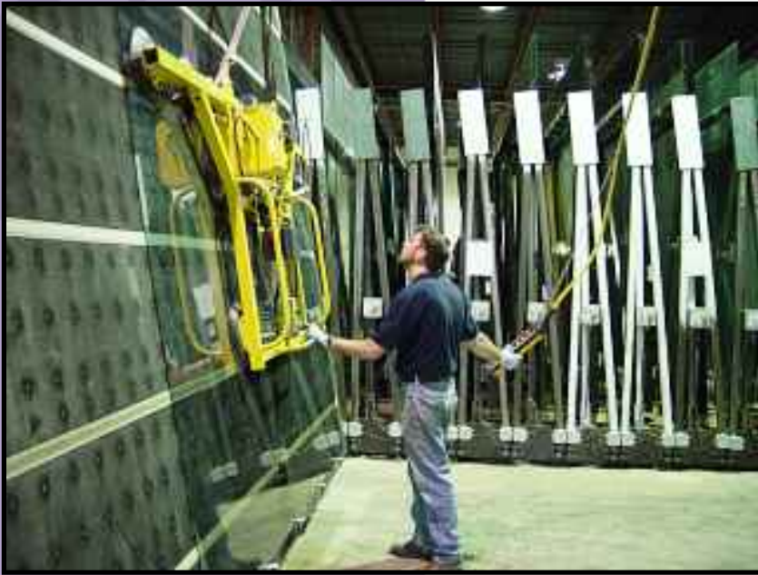
Garibaldi Glass employee Scott Wright uses a lifting frame with special suction cups to move large sheets of glass over to the cutting table.
